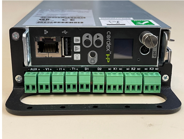
Figure 12: Alarm and signal connections
