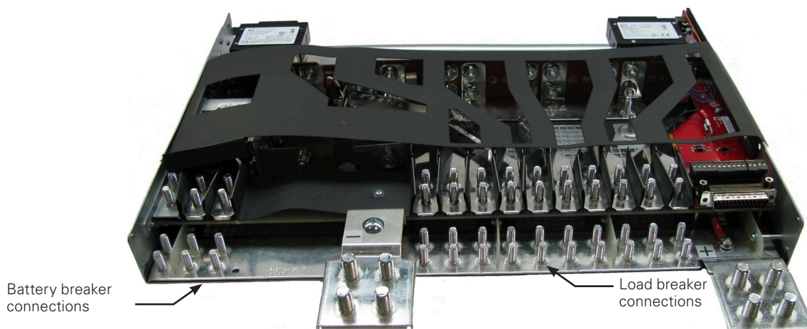
Figure 3: Cordex® CXDM-E1 distribution panel rear output connections
