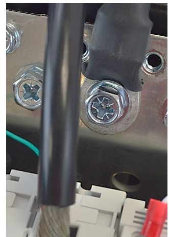
Figure 9 Connecting the battery
