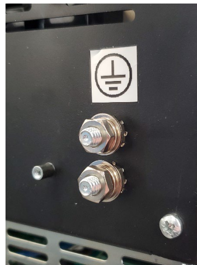
Figure 7A: External Earth Termination
