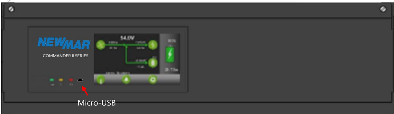
Figure 17: 3U EM4x-01 Front Panel micro-USB
