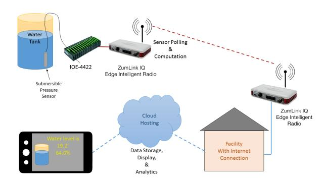
Figure 1: Facility Network Diagram
