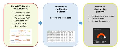
Figure 2: Process flow via Node-RED running on ZumLink IQ
