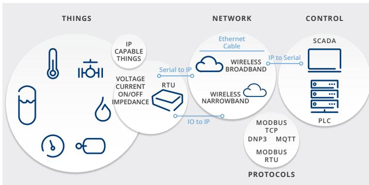
In this architecture, the serial interface from RTUs can be connected to “Serial to IP” adapters, which enables serial based IP accessibility via IP network. This approach can also be used for traditional SCADA master with serial interface.
