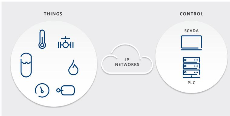
The architecture above works for green field deployment, meaning that if an operator wants to move to IIOT, they would need to upgrade all their existing sensors and other controllable equipment (machines) to IP capable “things”. This would be expensive. A more practical approach would be to reuse existing “things” by connecting them with IIOT adapters, and migrate to IIOT gradually.
