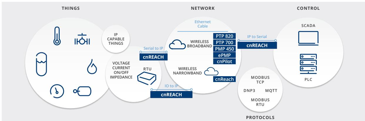
For operators with existing IP networks, the cnReach IO expander can be used to migrate the traditional “Things” to IIOT architecture. Operators can also deploy PTP820, PTP700, PMP450, etc. to transport the IIOT traffic if line-of-sight wireless broadband is feasible. In non-line-of-sight deployments, the cnReach narrow band radio can be used to enable the IIOT data transport.
