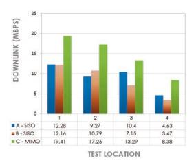
Figure 3 - SISO vs. MIMO Test Results [1].
