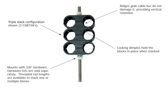
**Features:** Allows cable attachment by using 3/8" hardware (not included). Coax blocks are stackable to allow up to six runs of cable per tower attachment. Stronger than competitive brands in both vertical retention due to stiffening ribs, increased width and dimples.
